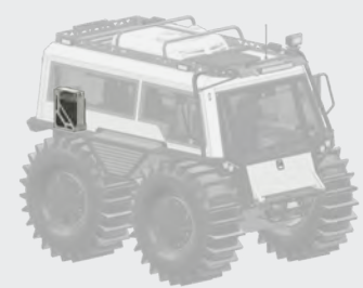
Additional fuel tank
